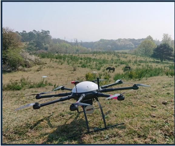
Picture: UAS LiDAR system used in re-wilded area of Mols Bjerge
