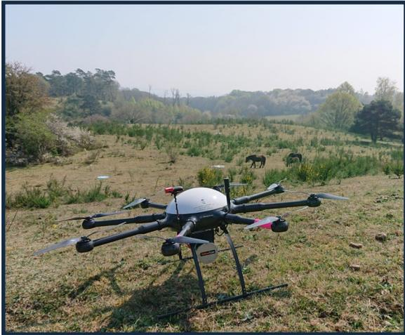
Picture: UAS LiDAR system used in re-wilded area of Mols Bjerger
